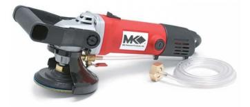
Like an Angle Grinder but with a built-in hose to dispense a steady stream of water while running. These use Velcro-attached 4 inch diameter Diamond Discs in 50, 200, 500, 1000, 2000 and 3000 grit as well as felt for polishing with Cerium Oxide.
