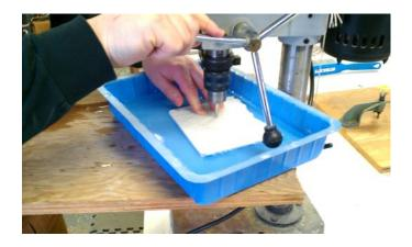
Drilling a piece of glass in a tray filled with water and a piece of styrofoam beneath the glass
