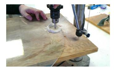
Drilling a large round of glass using putty to contain a pool of water as coolant.
